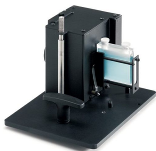
Figure 5: The ISA-220 integrating Sphere can measure cuvettes with a pathlength up to 50 mm
