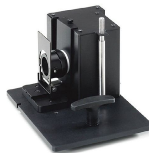
Figure 6: ISA-220 in Reflectance Configuration
