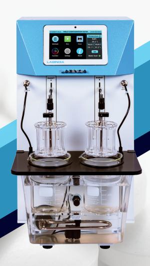
Disintegration test is intended to demonstrate the complete powder formation of the solid formulation. Labindia has introduced a novel Tablet Disintegration Tester for testing the disintegration time of tablets, capsules, and other solid dosage forms.
