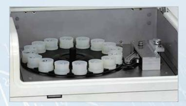
The automatic 16-positions sample changer coupled with the fast measurement increases the productivity of your lab up to 1000 samples per workday.
