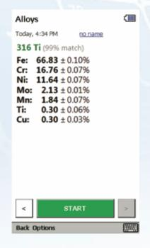
ProSpector 2 is a powerful handheld XRF analyzer, designed by Elvatech. Due to the advanced hardware and unique software algorithms, ProSpector 2 provides ultimate speed and accuracy of the elemental analysis. ProSpector 2 combines powerful analytical software toolkit with an easy-to-use interface, allowing even novice operators to perform any necessary measurements in seconds.
