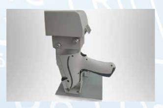
Use a laboratory stand to prevent X-Ray scattering when analyzing small objects or light matrix samples.
